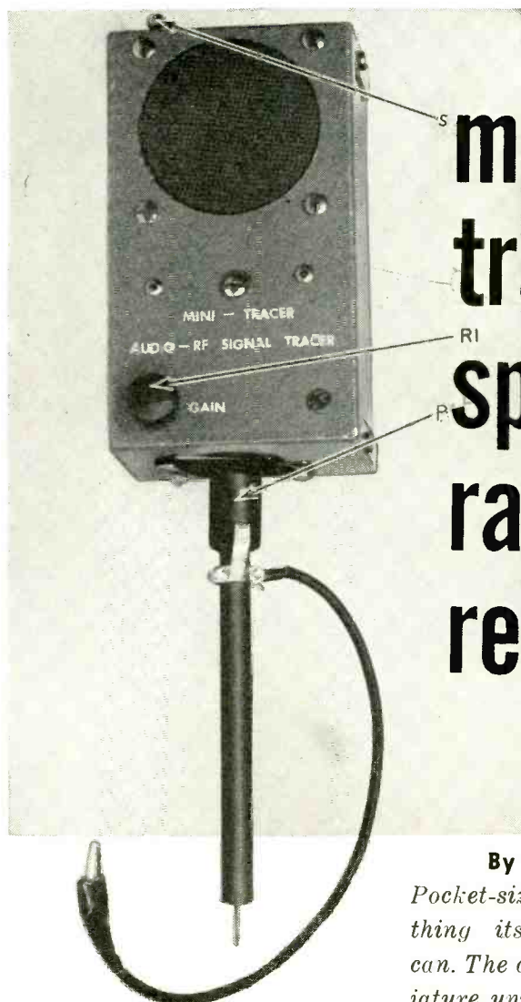
The completed unit with the rf probe attached.
