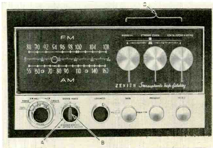
Zenith has extended stereo control (A) on panel of their hi-fi instruments. Clockwise rotation moves indicator from monaural to standard stereo (C). Balance control (B) is mounted coaxially with stereo range control.
