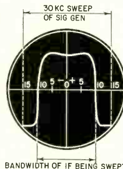
Fig. 4—Flat-top alignment for wide-band AM tuners for hi-fi radio reception.
